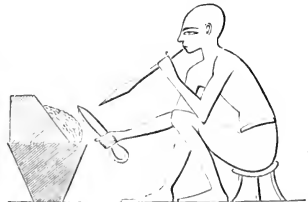
Egyptian Blow-pipe, and small fire-place with cheeks to confine and reflect the heat. (Wilkinson.)
