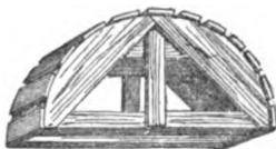
Centering of a Round-headed Arch.
