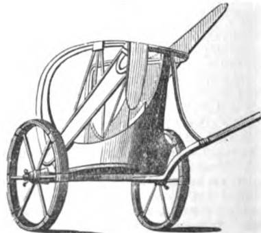
Ancient Egyptian Chariot, showing the method of attaching the Axle to the Wheels, to the Pole, and to the Body of the Car.
